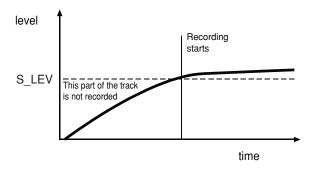
Conversely, you should be aware that if the sync level setting is too low, the noise level of an analog source may be higher than the sync level, so that sync recording fails to start.
